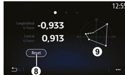
When you accelerate, slow down or turn, the vehicle undergoes transverse and longitudinal acceleration. This function can be used to see these and measure them in real time.
