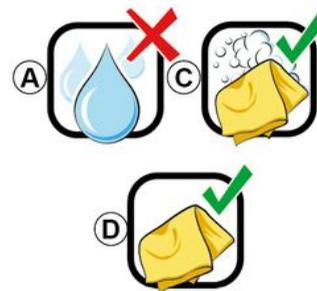
Wipe the screen gently using a clean, lint-free soft micro-fibre cloth moistened with soapy water.
