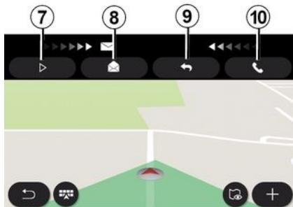
During driving, the SMS can be read by the multimedia system's synthetic voice by pressing "Play" **7** or you can return the contact's call by pressing the "Call" button **10**.
