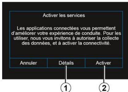
If the connected services are not yet activated, the multimedia system suggests that you send the activation request to the server by pressing "Connection", then confirm the request by pressing "Activate" **2**.
