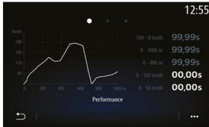
The measurement of performance is automatic and begins as soon as a speed above 0 mph (0 km/h) is detected. It is automatically reset once the vehicle has stopped for more than two seconds. The deceleration measurement begins during a significant braking.
