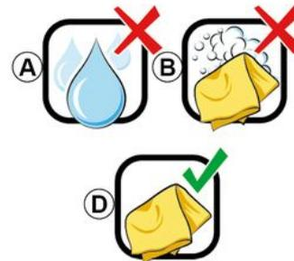
**Use only a clean, lint-free, soft dry micro-fibre cloth** to clean the touchscreen so as not to damage the anti-glare materials.
