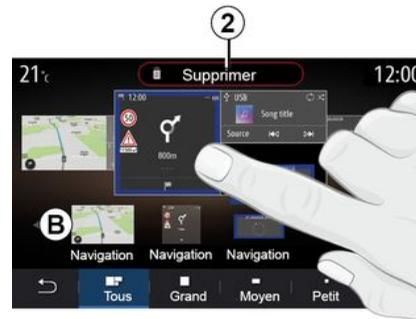
Press and hold the widget that you wish to delete. It changes colour to confirm the registration. Drag and drop on the "Delete" button **2** or slide the widget into zone **B**.
