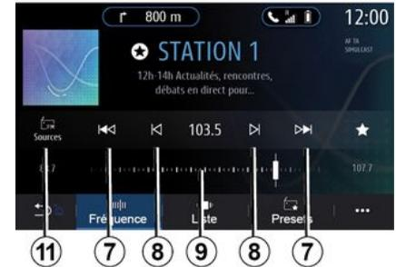
Use this mode to select radio stations by frequency in the radio band selected. To scan the frequency range, you have two options:
